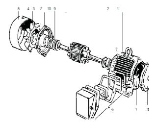
FIGURE 3. MAIN PARTS OF THE ASYNCHRONOUS ELECTRIC MOTOR
