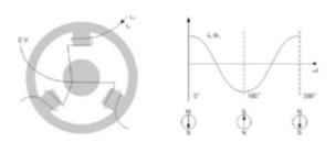
FIGURE 5. TWO-PHASE ASYMMETRICAL ROTATING FIELD
