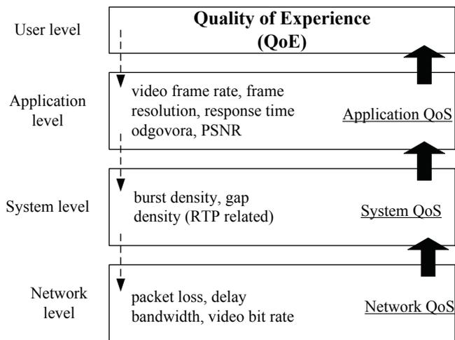
FIGURE 1. QoE AND THE LAYERED PROTOCOL STACK QoS, [16].
